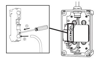
**3.** Connect the earth wire of the domestic system by pressing on the spring connection of the earth terminal with a screwdriver checking that the wiring has been done correctly.
