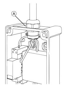
**1.** Choose either the pipe-box connector or cable-gland supplied, install it at position A and insert the power supply cables.
