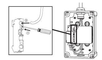
**3.** Connect the easyWallbox earth wire by pressing on the spring connection of the earth terminal with a screwdriver checking that wiring has been done correctly.
