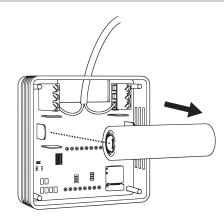
**4.** Remove the battery carefully and replace it with an equivalent one (AA **3.6** V).
