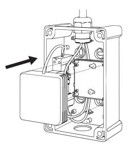
**3.** Reposition the gateway cover ensuring that the plastic supports are not damaged.
