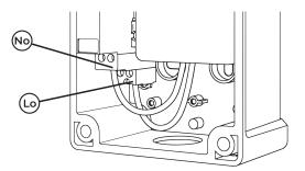
2. Connect the easyWallbox line cable (L) to the terminal indicated with <sup>①</sup> Lo and tighten the screw checking that the wiring has been done correctly. Connect the easyWallbox neutral wire (N) to the terminal indicated with <sup>①</sup> No and tighten the screw checking that the wiring has been done correctly.
