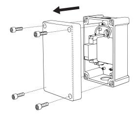
2. Remove the front cover of easyCounter by unscrewing the 4 screws.
