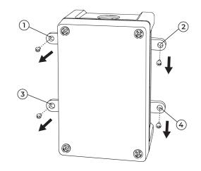
7. Loosen the screws fixing easyCounter to the wall.
