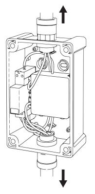
**5.** Loosen the connectors/cable-glands and remove the supply cable to easyWallbox and the domestic electrical system from its housing.
