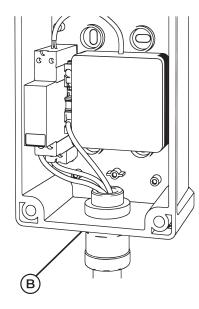
**1.** Use the pipe-box connector supplied, install it in position B and insert the power supply cables of the domestic system. Shorten the connection wires to the appropriate length (avoid leaving too much cable margin).
