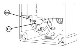
Connect line cable (L) of the domestic system to the terminal indicated with ↓ Lo and tighten the screw checking that the wiring has been done correctly.
