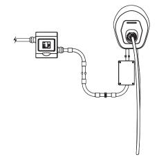
If **easyWallbox** has been installed in Plug & Play mode, **easyCounter** must be installed on the electrical line powering the socket for the connection of **easyWallbox**.
