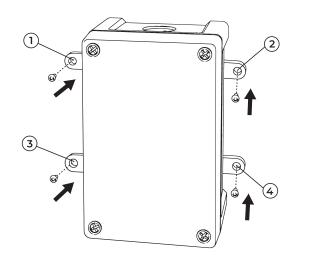
**5.** Position **easyCounter** in correspondence with the holes and fix it to the wall using the screws supplied.
