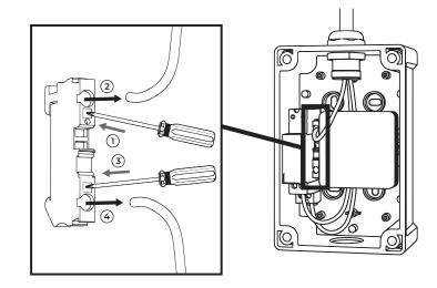
**4.** Disconnect the earth wire of easyWallbox and the domestic system by pressing on the spring connection of the earth terminal with a screwdriver.
