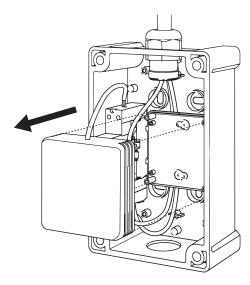
**1.** Remove the gateway cover by extracting it from its position.
