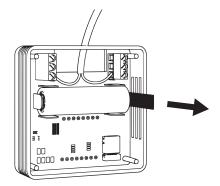
**2.** Remove the tab on the positive pole of the battery. Once removed, the gateway will start automatically.
