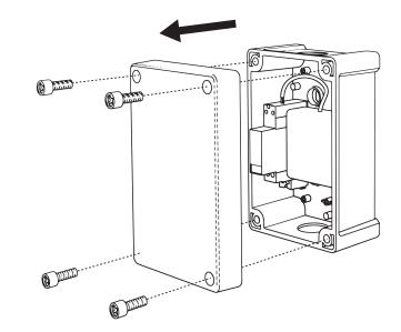
2. Remove the front cover of easyCounter by loosening the 4 screws.
