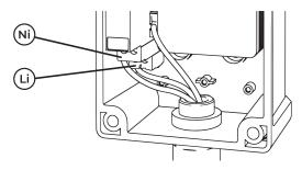
2. Connect the line cable (L) of the domestic system to the terminal indicated with  $\hat{1}$  Li and tighten the screw checking that the wiring has been done correctly.
