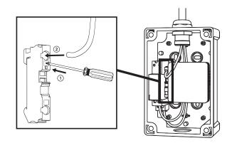
**3.** Connect the easyWallbox earth wire by pressing on the spring connection of the earth terminal with a screwdriver checking that wiring has been done correctly.
