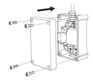
6. Reposition the front cover of easyCounter and tighten the 4 screws.
