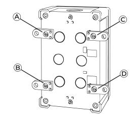
**1.** Position the wall brackets supplied in the kit and fix them in positions A, B, C and D with the appropriate screws.
