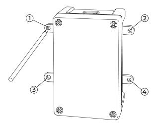
**2.** Place easyCounter in the desired position and mark the points for the holes on the wall.
