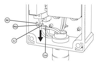
**3.** Loosen the screws on the terminals that the phase and neutral cables of the energy meter are attached to and remove them from the housing.
